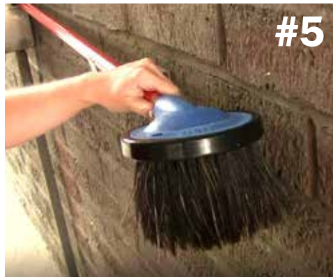
Step 5: Spin the brush to the right until you feel the cartridge catch the threads. Keep twisting until the cartridge is firmly in place. It helps to also push the cartridge while twisting. If properly inserted, the cartridge should stay in place without having to hold it anymore.
