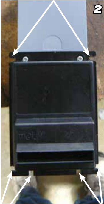
2 Use your Mars Validator for a pattern to cut in the mounting stud holes.
