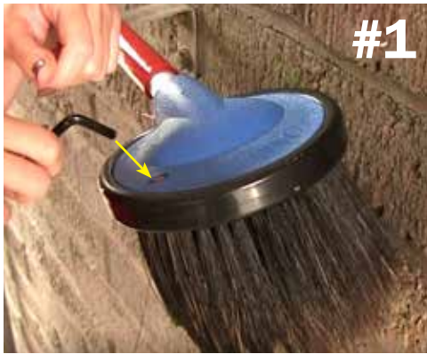
Step 1: Using an Allen wrench, give about two left twists to the hex screw. You only need to loosen it enough so the screw is no longer touching the cartridge.
