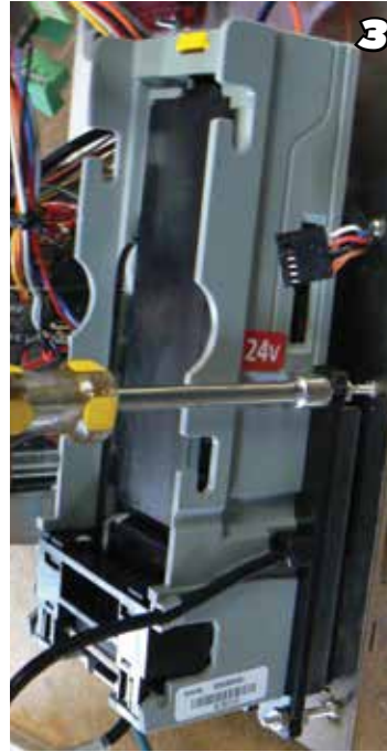
3 When ready to mount, use 6/32 flat head bolts and washers to attach your faceplate.
