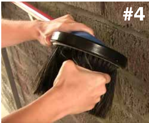
Step 4: Take your new or cleaned cartridge and grip the bristles the same way you did in step 2. Again, grab the handle or brush base with your other hand.
