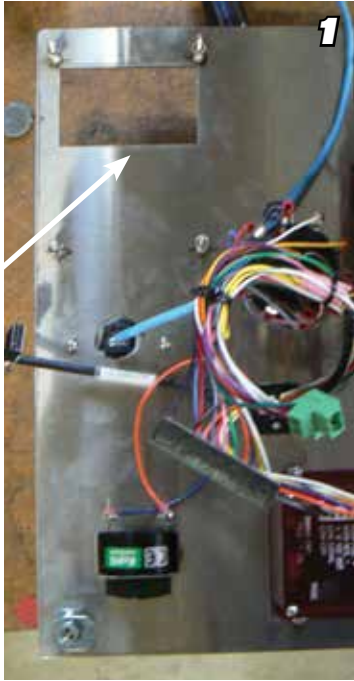
1 Your coinbox faceplate will need a hole measuring 3¼" W X 2" H for your validator. If you need to create the hole, make sure it is plasma-burned.
